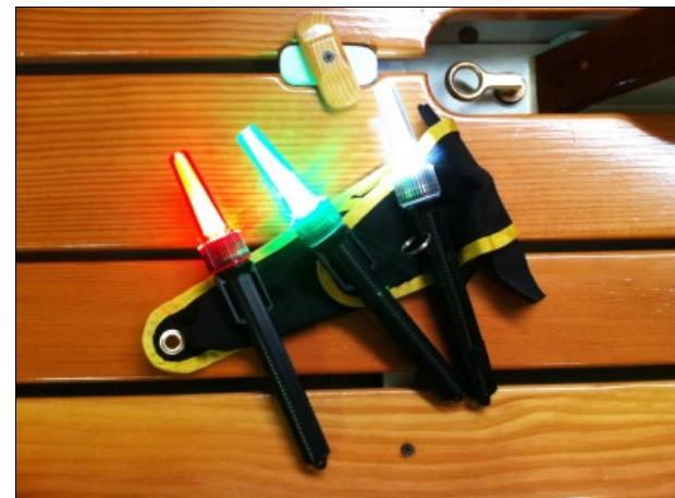
batteries, offering a listed burn time of over 50 hours. The LED bulbs have a 10,000-hour life and use about one tenth the power of an incandescent bulb. A pair of LEDs in each light illuminate a 2"-long white plastic insert in the lens that radiates the light in all directions. The red light has white LEDs, the green light has green LEDs.
